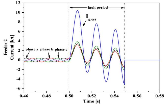
Fig. 4. Phase currents in feeder-2 and the zero-sequence current to the electrical ground of the ESS interconnecting transformer.
