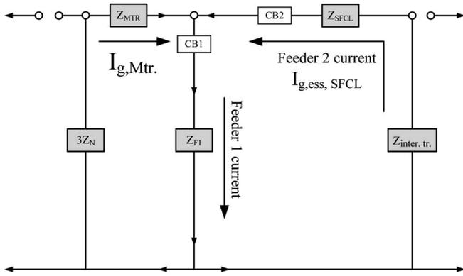
Fig. 8. Zero-sequence component of the equivalent circuit shown in Fig. 5.
