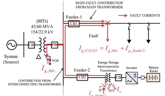
Fig. 2. Effect of a single line-to-ground fault on an ESS interconnecting transformer without an SFCL.
