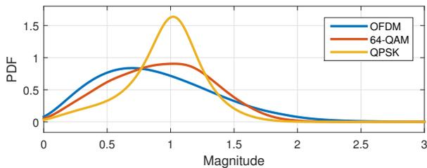
Fig. 6. Probability density functions (PDF) of the signal envelope for various modulation schemes, normalized to a root-mean-square magnitude of one.
