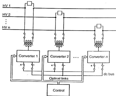
Fig. 1. General schematic of IPFC transmission line.
