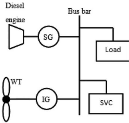
**Fig. 1** Schematic diagram of the proposed isolated hybrid wind-diesel generation system
