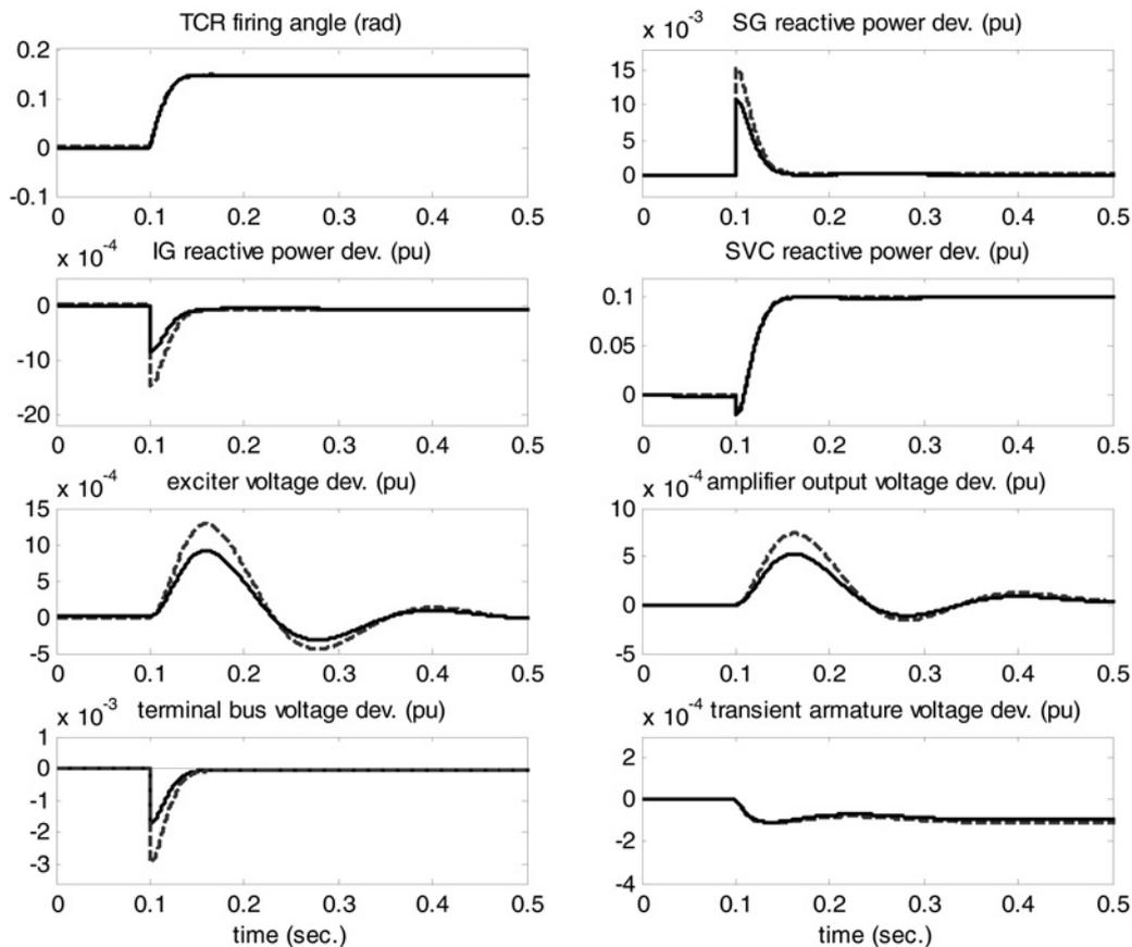
**Fig. 9** Simulation results of the proposed scheme with 10% step increase in load reactive power, with no change in input wind power, (— FMPC and - - - MPC)
