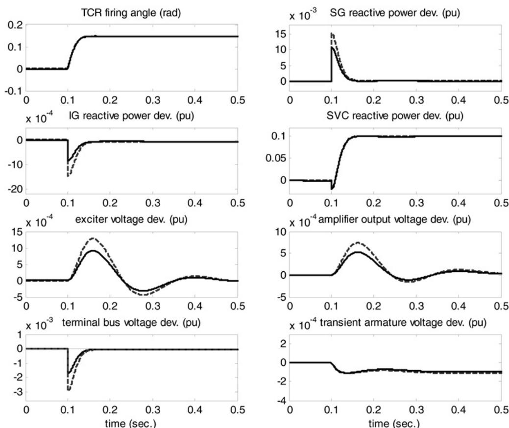
**Fig. 10** Simulation results of the proposed scheme with 10% step change in load reactive power with no change in input wind power, (— FMPC and - - - MPC)
