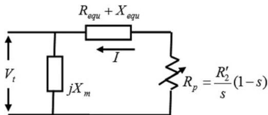
Fig. 3 Approximate equivalent circuit diagram of induction generator
