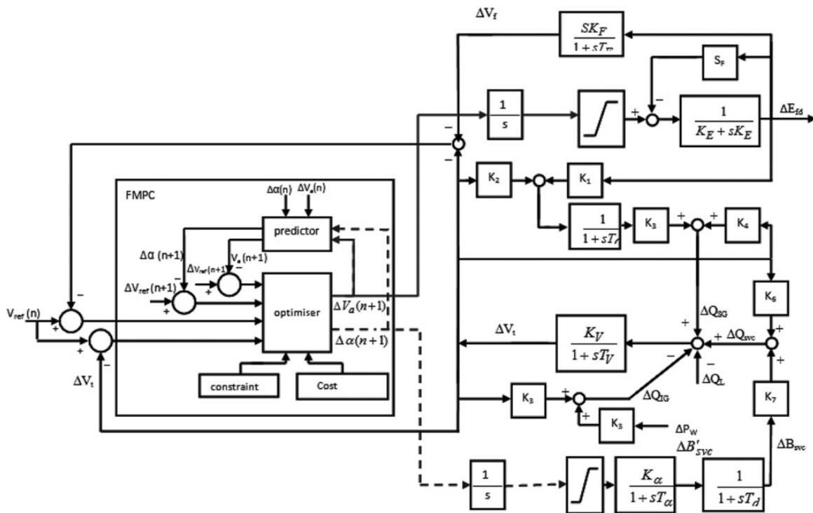
Fig. 7 Block diagram of the wind energy conversion system with the proposed FMPC controller
