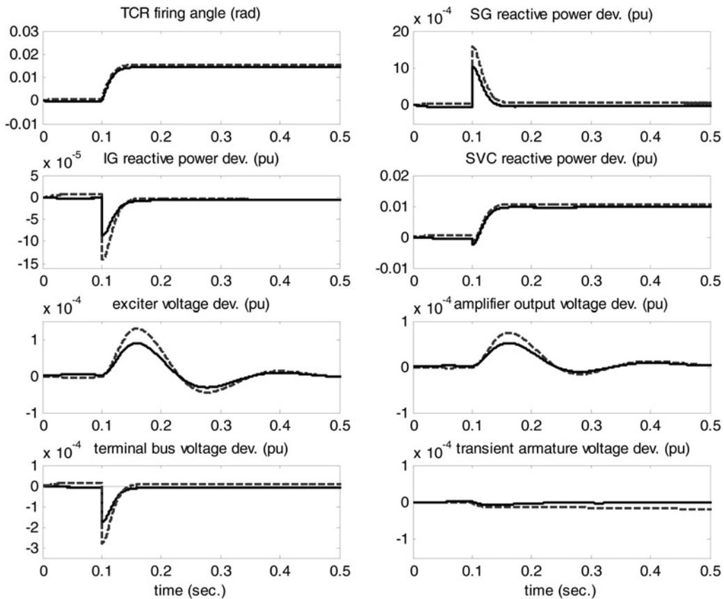
**Fig. 8** Simulation results of the proposed scheme with 1% step increase in load reactive power, with no change in input wind power, (— FMPC and - - - MPC)
