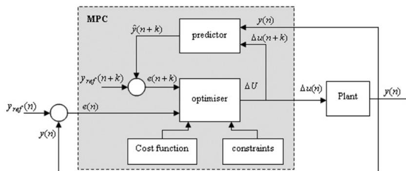
Fig. 6 Basic structure of MPC
