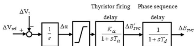
Fig. 4 Block diagram of the proposed small-signal thyristor-controlled SVC
