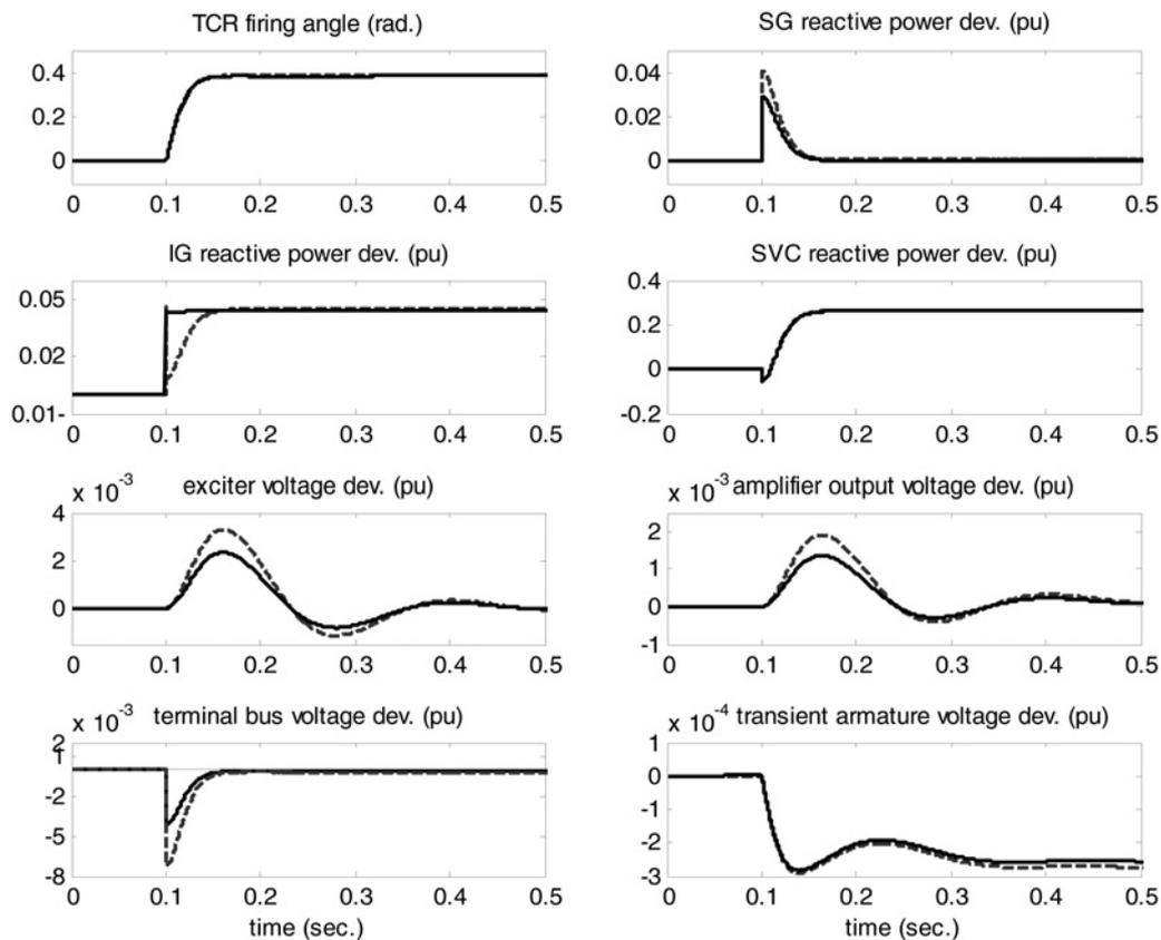
Fig. 11 Simulation results of the proposed scheme with 15% step change in load reactive power plus 10% step increase in input wind power and parameters changes, (— FMPC and - - - MPC)
