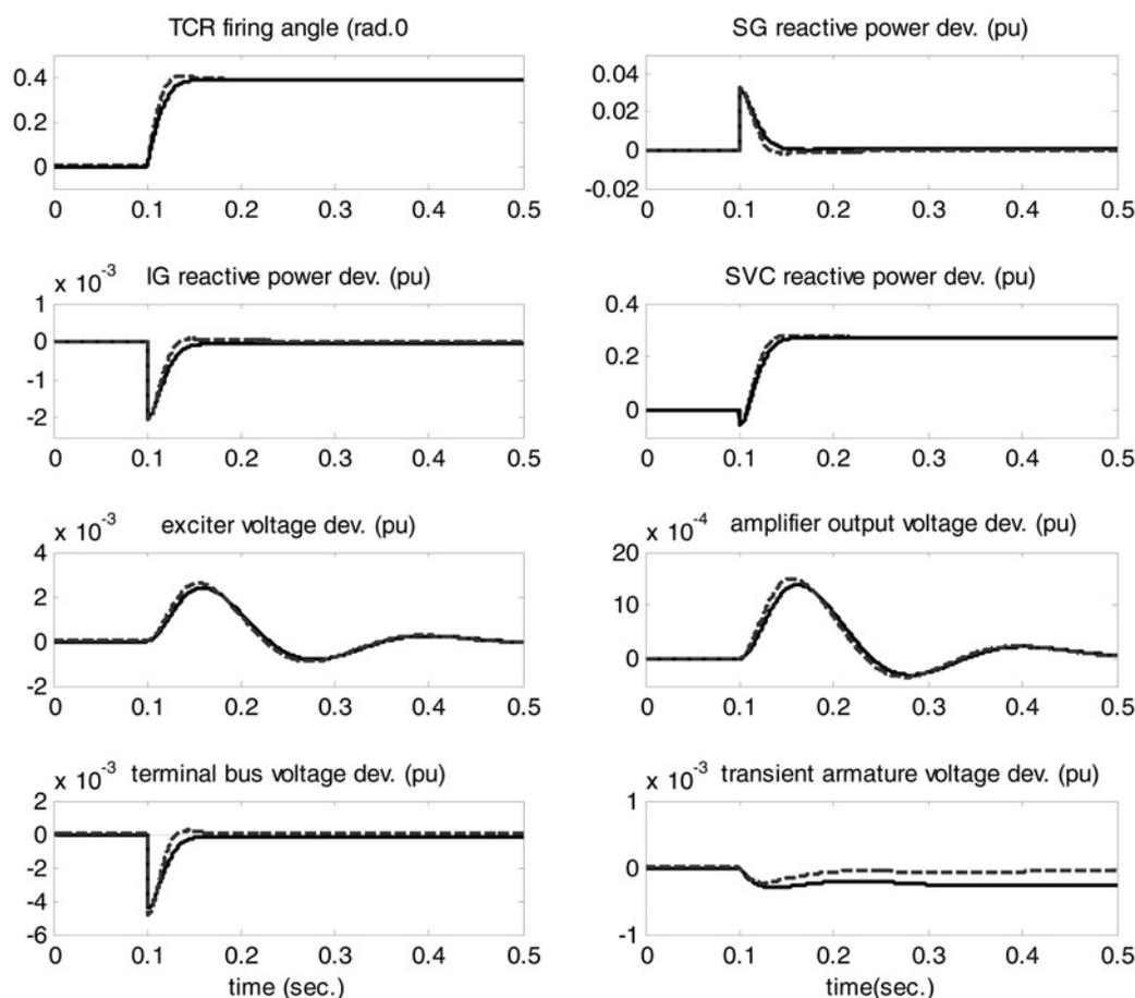
**Fig. 12** Simulation results of the proposed scheme with 15% step change in load reactive power with no change in input wind power, (— FMPC and - - - MPC)
