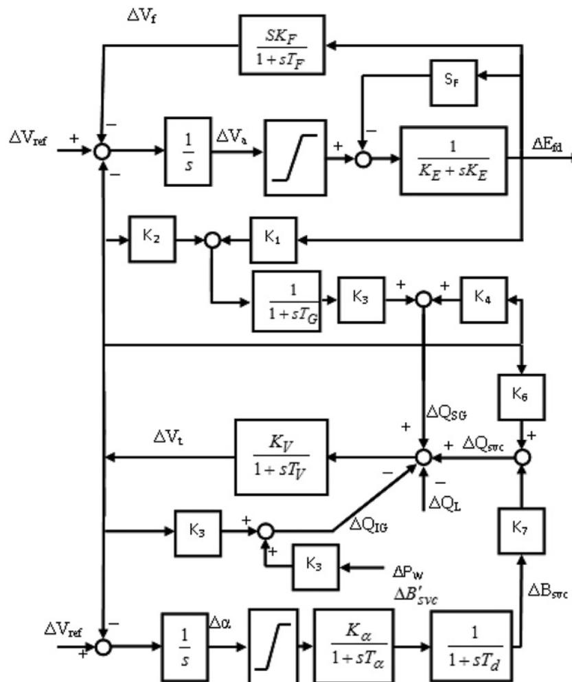
Fig. 5 Transfer function block diagram of the hybrid wind–diesel system
