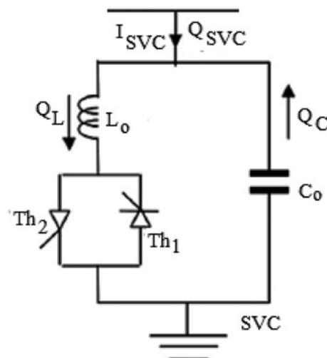
**Fig. 2** Block diagram of SVC
