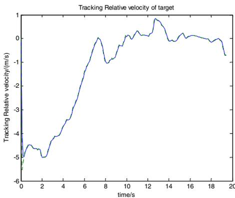
Fig 2. Relative velocity and its tracking output signals
